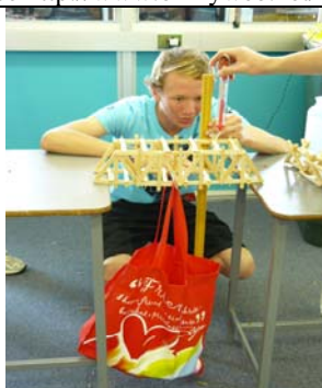
Ben Wreide Year 12 Engineering Technology class – made this bridge from paddle pop sticks and toothpicks which held a weight of 12.25kg with a 5mm deflection.
